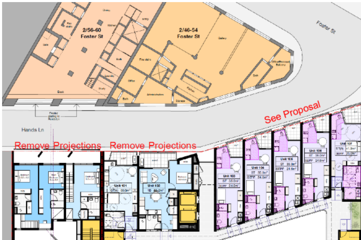
Figure 48: Illustrating the removal of balcony projections opposite residential uses, and retention of balcony projections opposite 46-54 Foster Street
